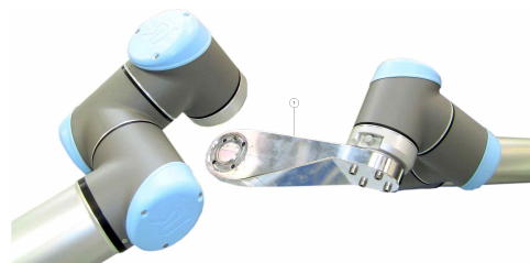
Calibration Connector attached to the Leader robot's tool flange and the Follower robot's tool flange (step 5).
